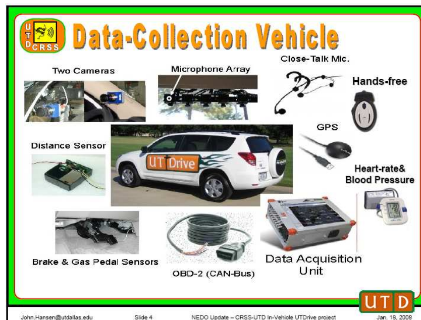
Figure 1: Data collection vehicle and the applied sensors in UTDrive Project
