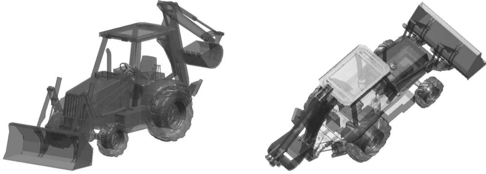
Figure 3.14: Backhoe model used in Xpatch scattering predictions. The view to the right corresponds approximately to the images in our experiments.
