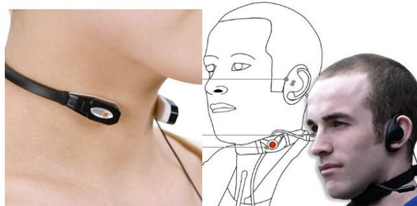
**Figure 1.** Conceptual designs for the proposed wearable mobile device using SSI together with auditory feedback
