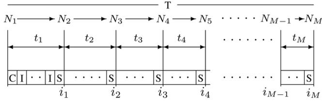
Fig. 1. Timing diagram of the operation of the system.  $S$ ,  $I$ ,  $C$  represent success, idle, and collision events, respectively.
