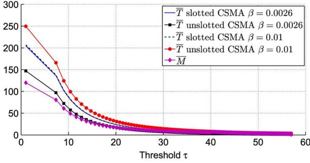
Fig. 2. Expected value of  $M$  and  $T$  with respect to threshold  $\tau$ .
