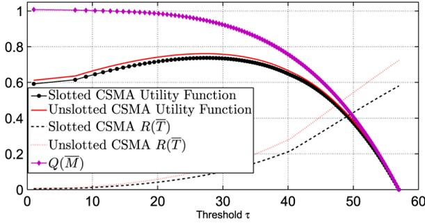
Fig. 3.  $Q(\bar{M})$  and  $R(\bar{T})$  with respect to threshold  $\tau$ , and corresponding overall concave utility function.
